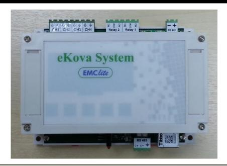
The ekoLITEs are multi-function controllers for monitoring, control and data logging. Its simple and yet versatile design ensures reliability and scalabilities. Each ekoLITE is capable of high level and low level interfacing to other third parties equipment to provide seamless operations.
